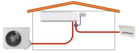
2. Wiring from circuit board to outdoor unit to indoor unit (normally on big size AC)
