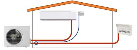
In both cases need to ensure current transformer is connected to the feed from circuit breaker as follows (only to LIVE):
